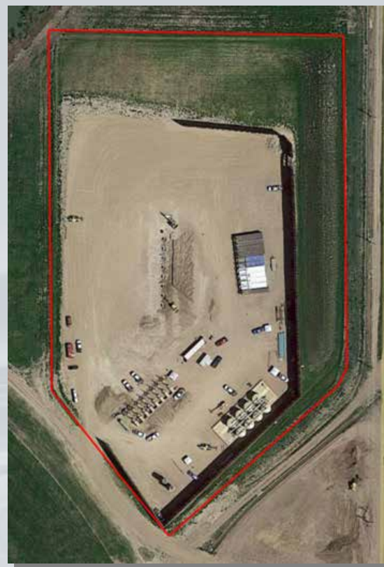
Figure 19: Bayswater's interim reclamation efforts reclaimed 7.3 acres on this specific location with the red line showing the original pad footprint.
